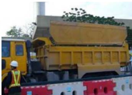
Cover dump trucks with mechanical shields
