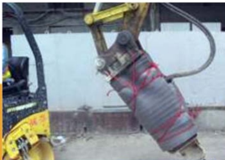
Acoustic jacket wrapped around hydraulic breaker
