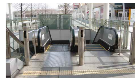
3.1.6.1h Tactile warning strips and audible signals at escalators
