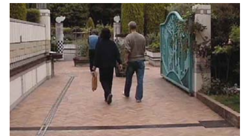
3.3.7.1h Clear visual and tactile clues leading to the entrance gate of the garden
