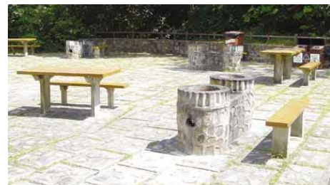
3.4.1.14b Accessible fire pit and picnic table with fixed seats and space for wheelchairs
