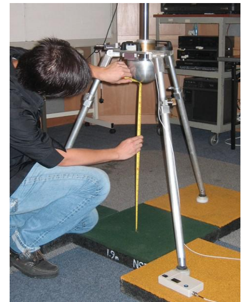
3.4.2.4 h Selection of an appropriate ground surfacing with impact attenuation quality is based on its performance (as shown here) but not the nominal thickness of the mat itself
