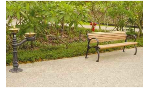
3.4.1.9 a Seating bench with armrest and backrest, and an adjacent wheelchair space
