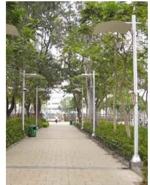
3.4.1.4b Access routes with lamp poles cleared from the walking surface
