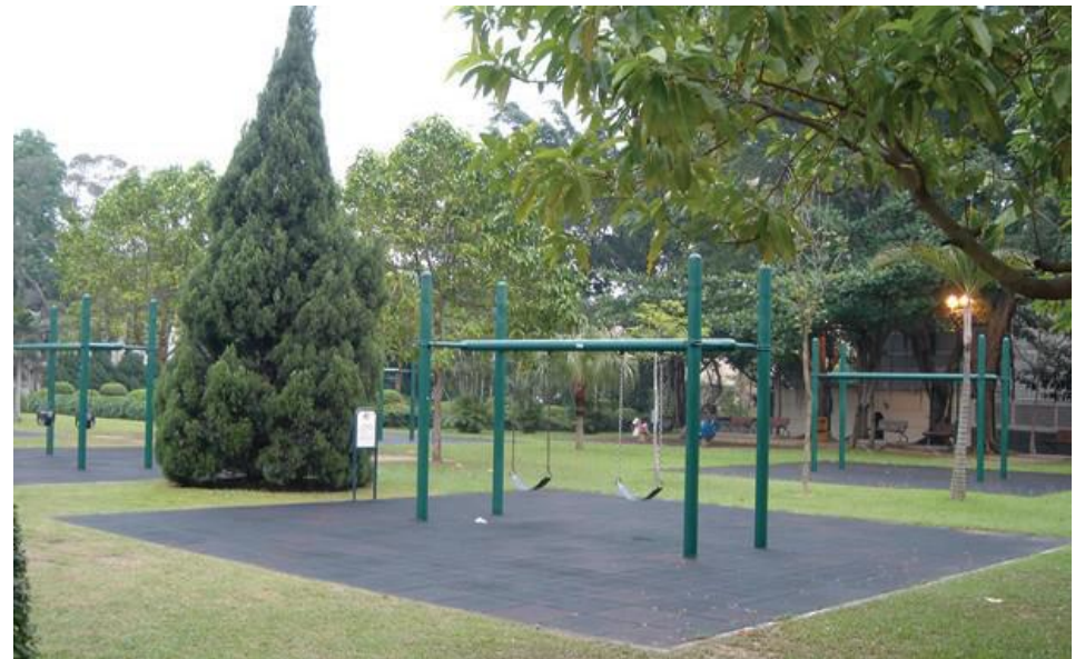
3.4.2.4 b The dimensions and configuration of the use zone/impact area is dictated by the type of play equipment. Swings take up a relatively large space for safety margins
