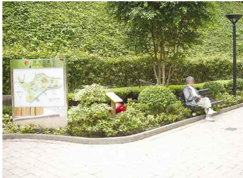
3.4.1 a Map, fire hydrant, seating bench, lamp pole are all recessed into the planter area
