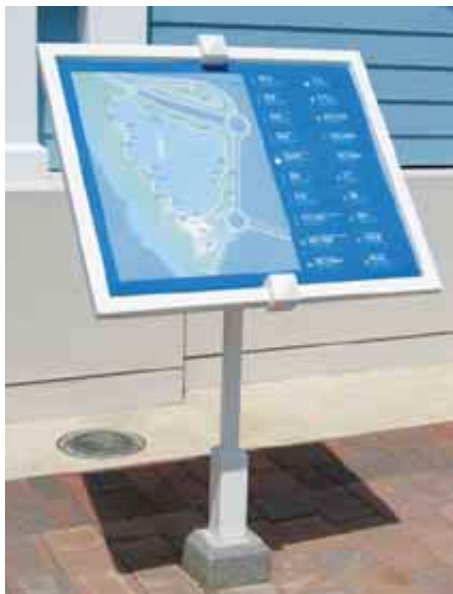
3.5.3a Directory with ordinary text and Braille giving information on the services and facilities
