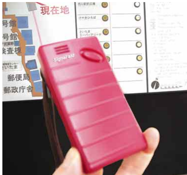
3.5.5.2b A voice information system that uses electric signboards to transmit signals to a portable terminal
