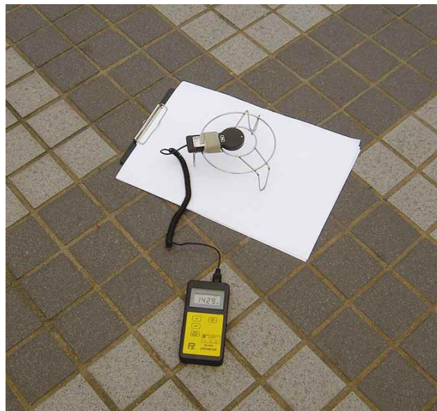
3.7.5.2a White paper is used to obtain data (Ln lux), which is compared with the readings (L lux) taken on the test surface
