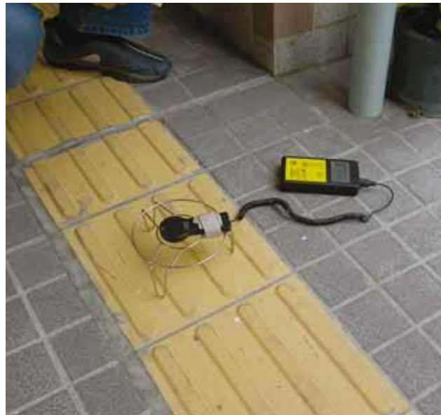
3.7.4.1a Using light meter to obtain data readings
