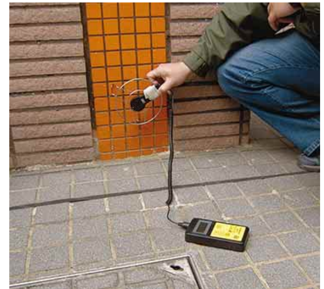
3.7.4.1b Field readings of different surfaces in external areas
