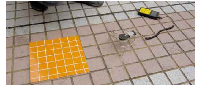
3.7.5.1a Readings of the light meter taken on two adjacent test surfaces
