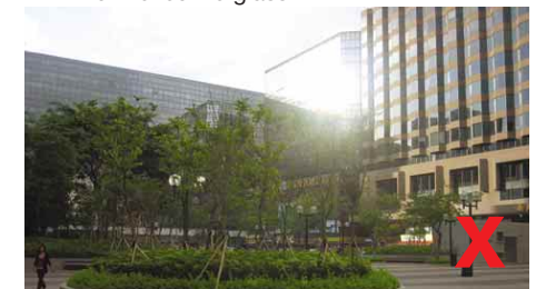
3.8.5.2b Reflected sunlight from a curtain wall building creates glare to a nearby garden
