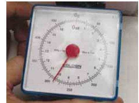
vi) Record the reading of the scale as the Pushing Force
