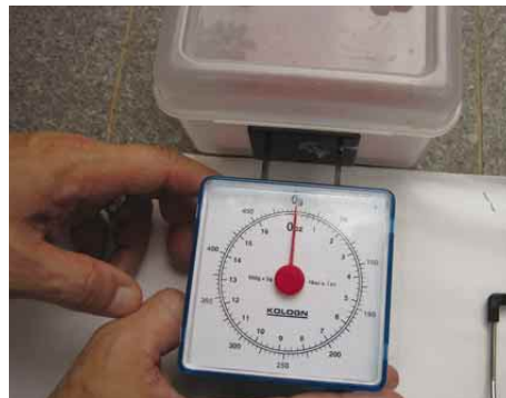
iv) Place the heel tap test box on the levelled flooring material to be tested and set the scale at zero against the front of it
