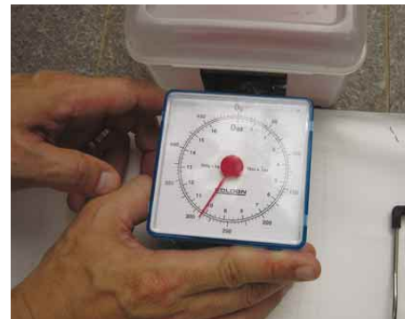
v) Push the scale towards the heel tap test box, increase the force gradually until it just starts to move
