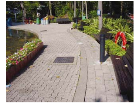
4.4m Furniture recessed from the walkway and a floating device provided near water areas for safety
