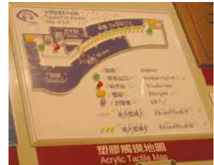
4.5q Tactile fire escape map that can serve a wide range of users
