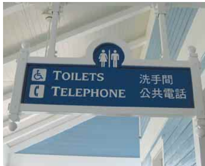
4.5n Signage with standardized pictograms in contrasting colours with the surrounding surfaces
