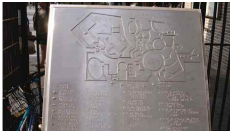
A2.4.1a Entrance map with tactile layout of the area and information in Braille
