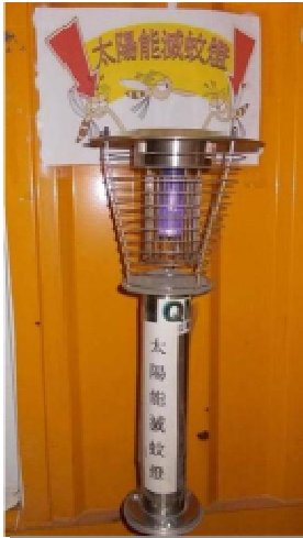
Photo 19. Mosquito killing device with solar energy panels
