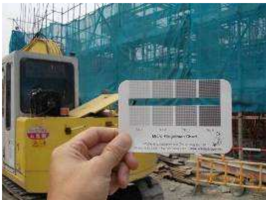
Photo 4. Black smoke monitoring was conducted by using Ringelman chart continuously for 30 seconds
