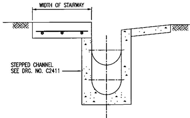
**CROSS SECTION OF COMBINED STAIRWAY & STEPPED CHANNEL**
