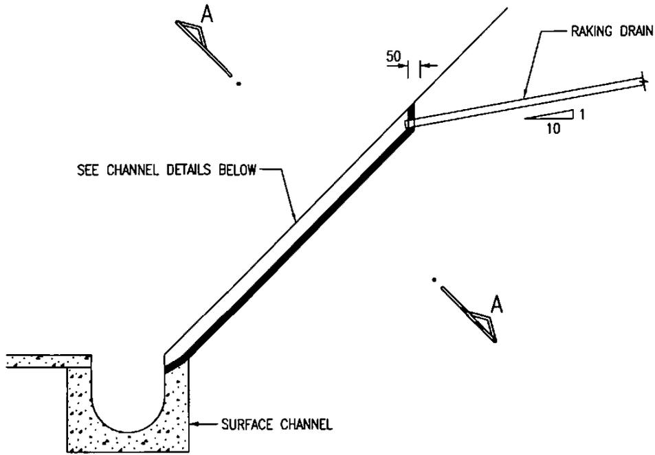
**SECTION THROUGH CONNECTING CHANNEL**
