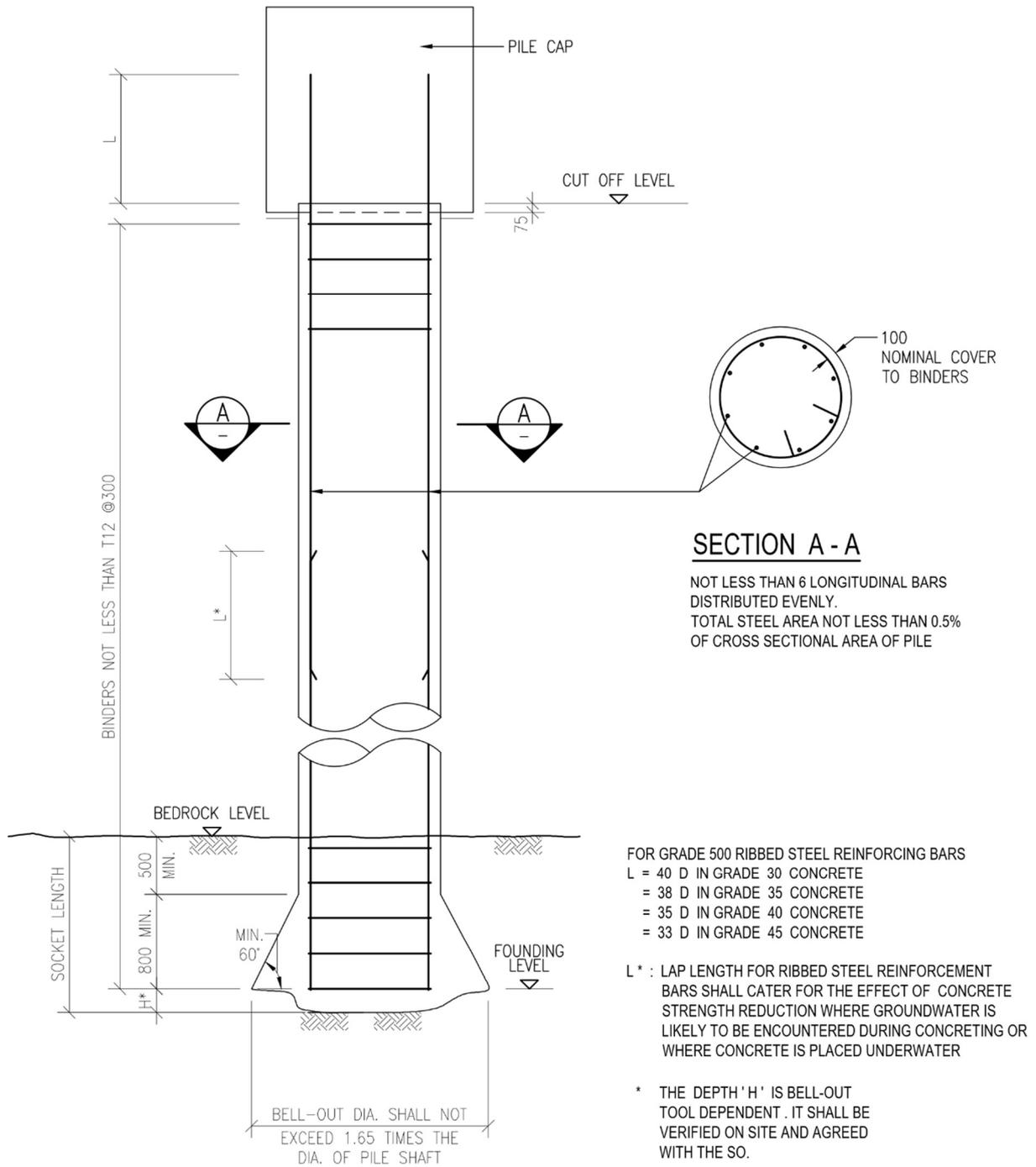
**TYPICAL DETAIL OF LARGE DIAMETER BORED PILE WITH BELL-OUT**
