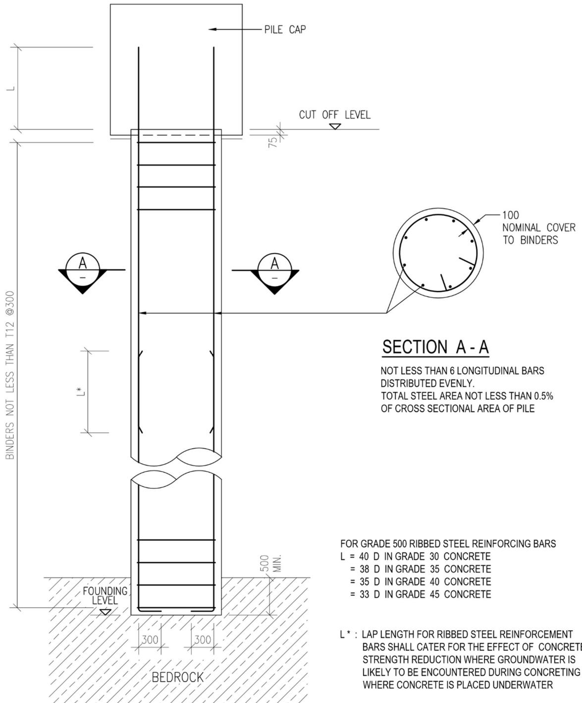
**TYPICAL DETAIL OF LARGE DIAMETER BORED PILE**
