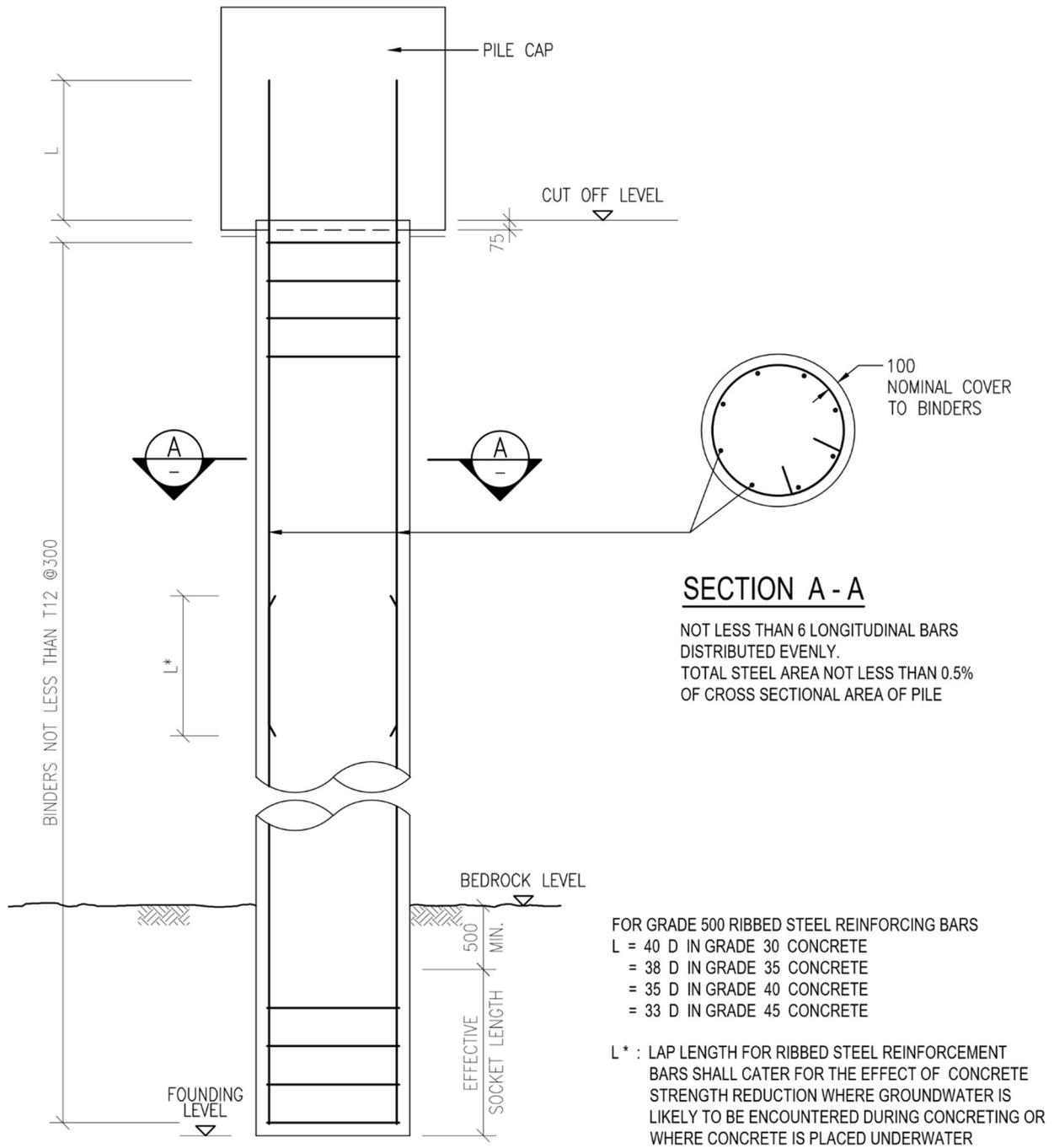
**TYPICAL DETAIL OF LARGE DIAMETER BORED PILE
