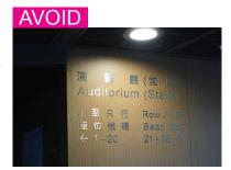
[Fig. D1.4] Signage with reflective surface can cause glare and should be avoided.
