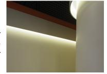
[Fig. D4.2] Indirect lighting which points at ceiling or wall surface should be considered to avoid direct exposure of eye to the light source.
