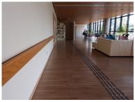
[Fig.D2.2] Handrails in high visual contrast against the background can help individuals with visual impairment to locate the handrails.
