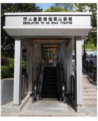
[Fig. B1.1] A weather protected escalator should be considered if there is substantial level difference between street and building levels.
