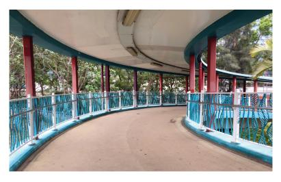
[Fig. B6.3] Curved ramp can be a sculptural architectural feature but it shall be designed to ensure safety and ease of use.
