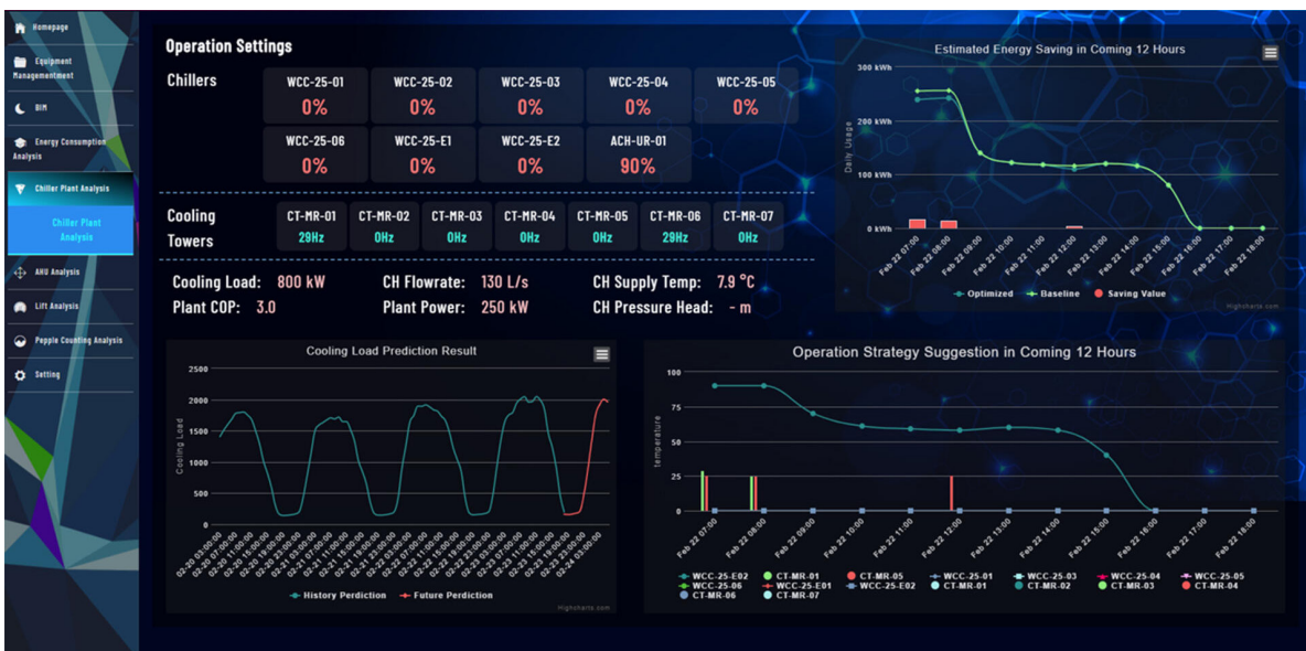
Illustration of Chiller Plant Optimisation Dashboard
