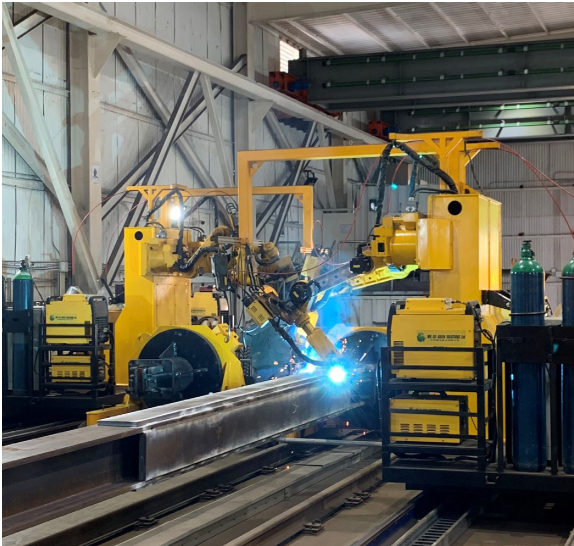
Automated Welding Robot
