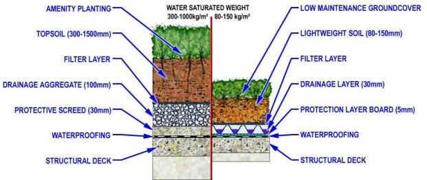
(Source and copyright <sup>©</sup> Urbis Ltd., 2006, adapted from drawings from Greenlink Küsters Ltd.) Note: Intensive green roof weights of 300-1000kg/m<sup>2</sup> refer to the most shallow soil depth needed for amenity groundcover or lawn grass (300mm). A soil depth conducive for successful tree growth (1500mm deep) is likely to weigh around 3300kg/m<sup>2</sup>, excluding the weight and wind-loading pressure of the trees.
